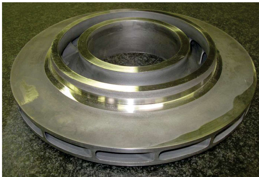
Fig. 1 — Impeller for gas compressor made by PM HIP from Ti-6Al-4V alloy powder. Courtesy of LNT PM Inc.
