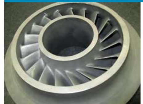
PICTURE 1B: Gas compressor impeller made by PM HIP from Inconel alloy 625 powder.
