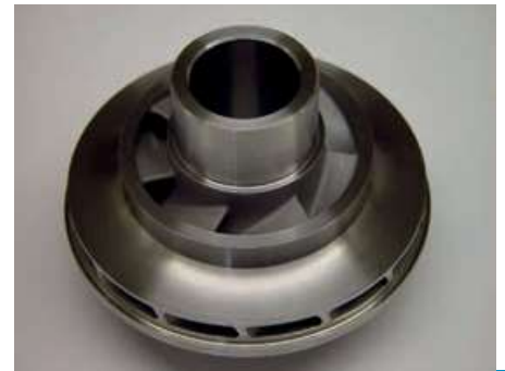
PICTURE 1A: Gas compressor impeller made by PM HIP from Ti-6Al-4V alloy powder (A).
