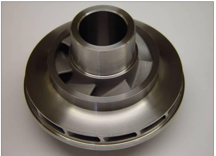
Figure 1A: Impeller made by PM HIP from Ti-6Al-4V alloy powder (A) (Source: LNT PM).
